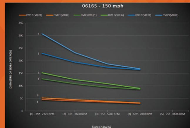
TESTES REALIZADOS COM PÁS DE 90mm EM TÚNEL DE VENTO (AERIAL APPLICATION TECHNOLOGY RESEARCH: COLLEGE STATION, TEXAS)
