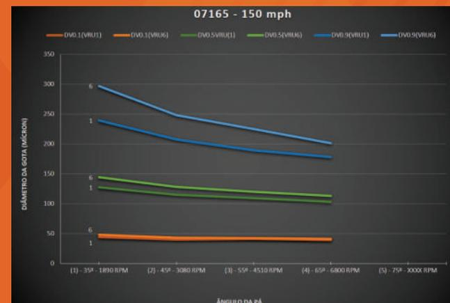
TESTES REALIZADOS COM PÁS DE 70mm EM TÚNEL DE VENTO (AERIAL APPLICATION TECHNOLOGY RESEARCH: COLLEGE STATION, TEXAS)
